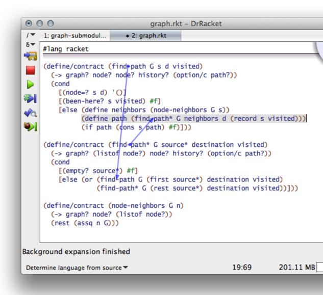
In contrast, submodules act exactly like plain modules when it comes to contract boundaries. Like define/contract, a submodule establishes a contract boundary between itself and the rest of the module. Any value flow between a client module and the submodule is governed by contracts. Any value flow within the submodule is free of any constraints.
