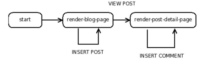
Each node (bubble) in this diagram corresponds to a request-consuming handler. As you might expect, we'll be using send/suspend/dispatch some more. Every arrow in the diagram will be realized as a URL that we generate with embed/url.
